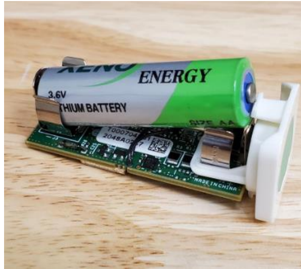
Figure 2-6: Battery Polarity Orientation
