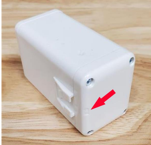
Figure 2-11: Proper Replacement Orientation of the Battery Cover
